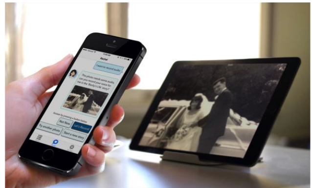
Figure 1. ReminX platform, shown on caregiver’s mobile device and on patient’s tablet. There is no interface for the patient to learn - simply picking up the tablet starts the stories and putting it down stops them. The tablet uses inductive charging, and while on its dock, acts as a photo frame showing all the photos in the system.
